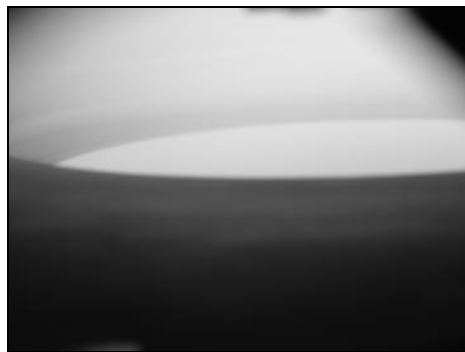
Figure 2.10: The white 6" target is engulfed in an Argon gas RF-plasma.
